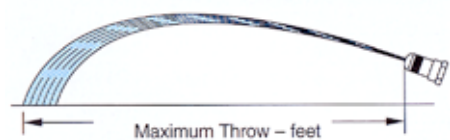
TIP SETTING "B" STRAIGHT STREAM SPRAY PATTERN
